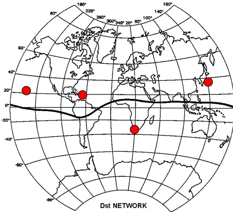
The **Dst index** gives the average (in longitude) **depression of the horizontal component in low latitudes (due to the ring current)**, which is proportional to the total kinetic energy of the particles injected and trapped in the Van Allen (electron) belt.
